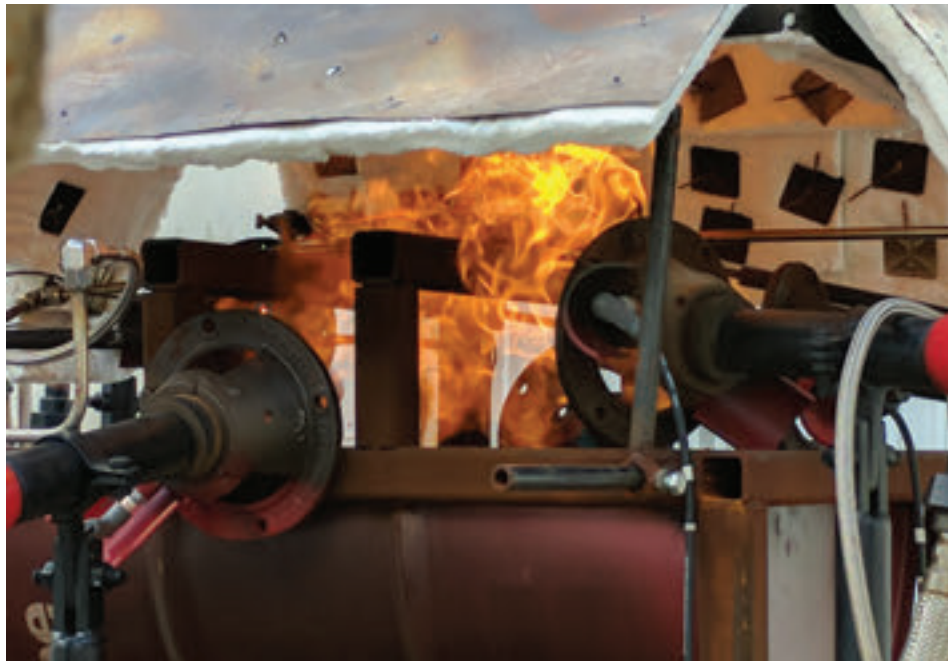
Fire safe testing to API 607, January 2017
